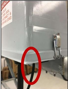
The black cable going to the satellite antenna *should not* be disconnected. The cable may be slipped through the bottom of the tower box. Ideally, it should be wedged through a seam in the tower box gasket as pictured to the left. Once the wire is in place, snap the tower box closed over the wire.
