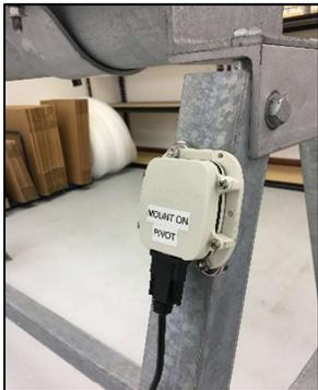
The satellite antenna should be magnetically mounted to the pivot’s steel structure **with the cord connector facing down**. The antenna should be unobstructed from a clear view to the sky. Do not place directly under the tower box or other equipment such as booster pumps. Avoid placing directly next to high voltage wheel motors wires.
